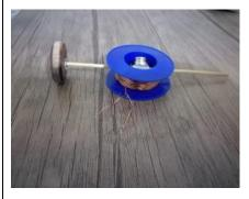
A bobbin was wrapped around the neodymium magnets, and when the magnets rotate, an induction current occurs.
