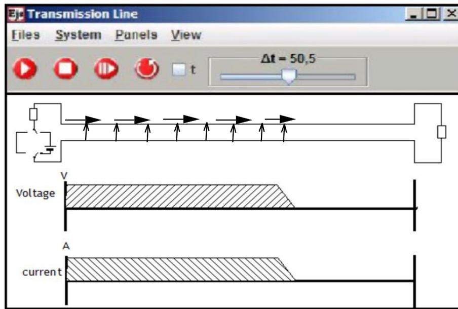
**Figure 7.** Transition Processes along a Parallel Circuit (Conductive Region between both Conductors Plus Load)
