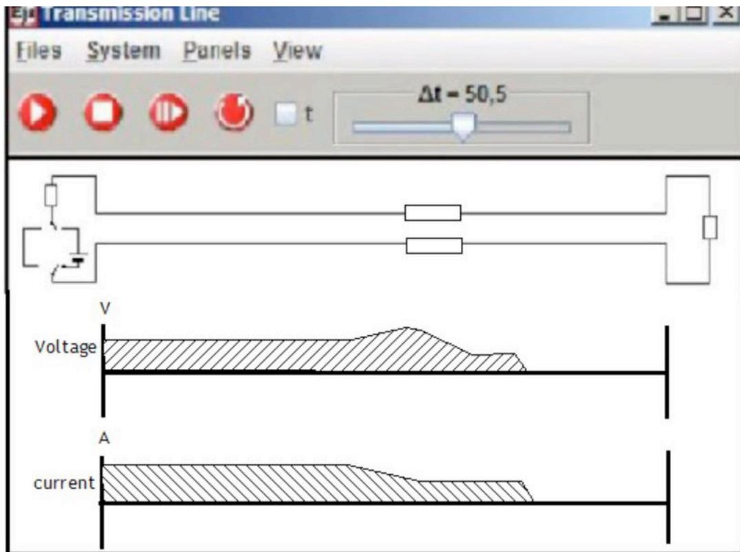
**Figure 6.** Transition Process for a Serial Circuit (Resistors on Both Lines Plus Load)
