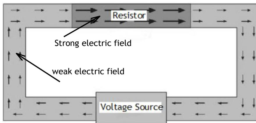
**Figure 2.** *Different Fields Inside the Conductor Wire and the Resistor*
