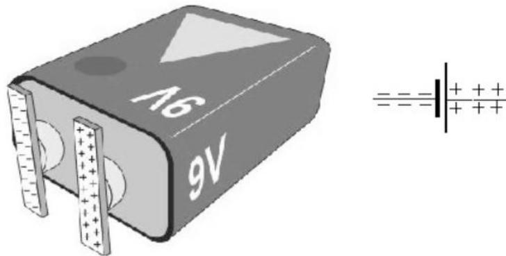
**Figure 8.** A Battery as Voltage Source with Surface Charges on its Metallic Outlets
