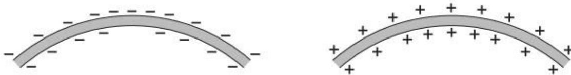
*Figure 7. Distribution of Surface Charges on Curved Conductors (Qualitative)*
