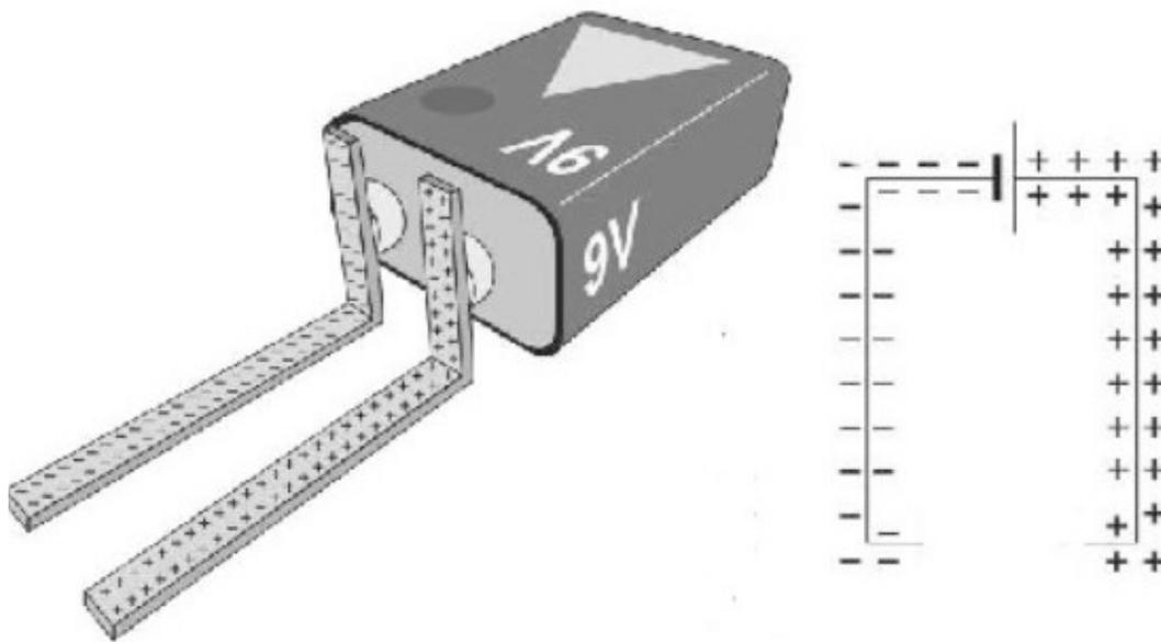
**Figure 9.** Power Source with Connected Conductors and Surface Charges
