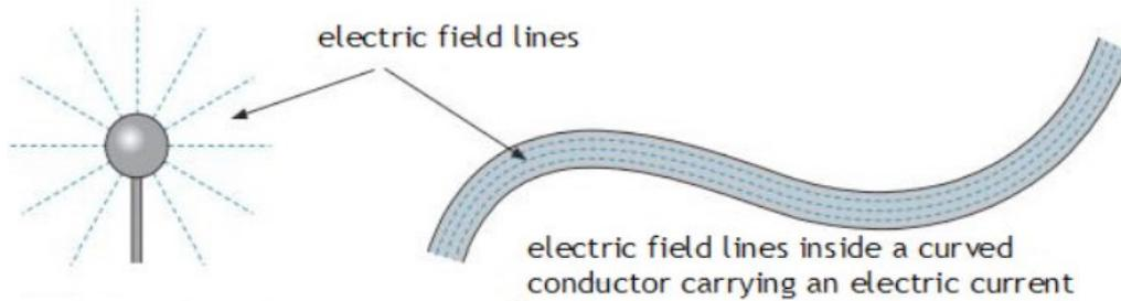
**Figure 3.** Spherically Symmetric Electric Field of a Single Charge Carrier  $\sim 1/r^2$  (left); Distance-Independent, Constant and Axially Aligned Electric Field Inside an Arbitrarily Curved Conductor (right)
