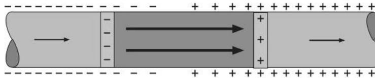
**Figure 4.** Charged Separating Layers between Resistor and Conductor
