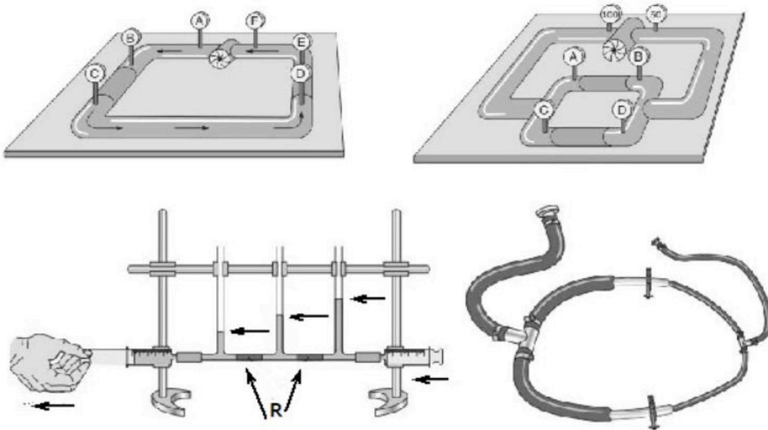
**Figure 11.** Figures and Instruments Used to Explain the Analogy between the Flow of Water and the Flow of Electrons
