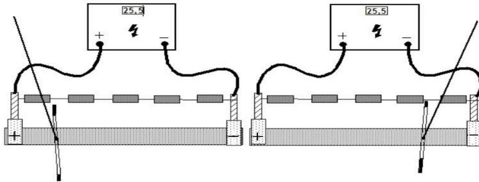
**Figure 13.** Interaction between a Current Carrying Chain of Resistors and a Straw Charged with Different Charges at Both Ends to Demonstrate the Existence of Surface Charges (<http://www.astrophysik.uni-kiel.de/~hhaertel/PUB/straw.flv>)
