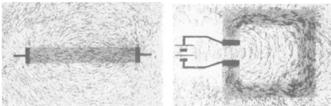
**Figure 12.** *Electric Fields Inside and Outside Differently Formed Resistors, Visualized by Scattered Grass Seeds (Jefimenko, 1962)*
