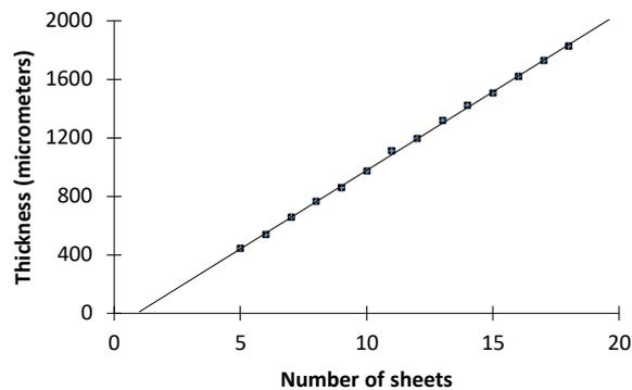
**Figure 3.** The thickness of different stacks of paper sheets. The dots are the experimental values determined by the coil and the line represents the linear fit  $Th \text{ (}\mu\text{m)} = 107.4 x - 97.1$
