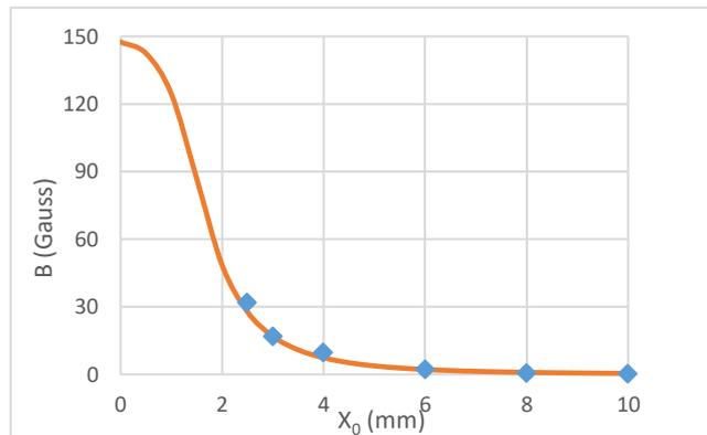
**Figure 2.** Variation of the calculated magnetic field given in eq. (9) with the distance (red line). Blue dots represent the experimentally measured magnetic field
