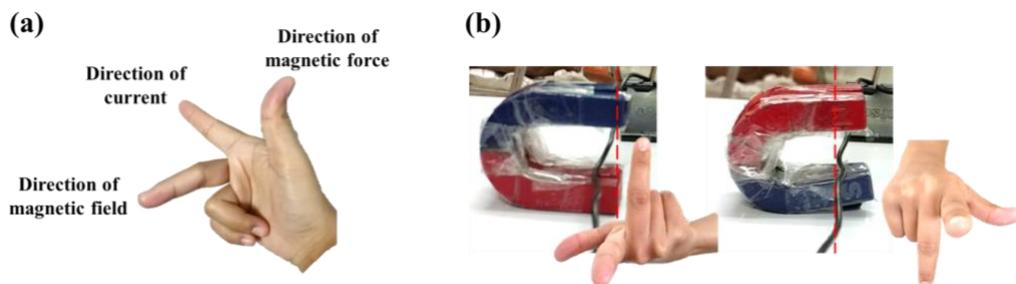
**Figure 4.** Underlining principle of magnetic force. (a) Fleming's right-hand rule to illustrate the magnetic force, current, and magnetic field (b) Wire moved in opposite direction when reversing the direction of magnetic field.
