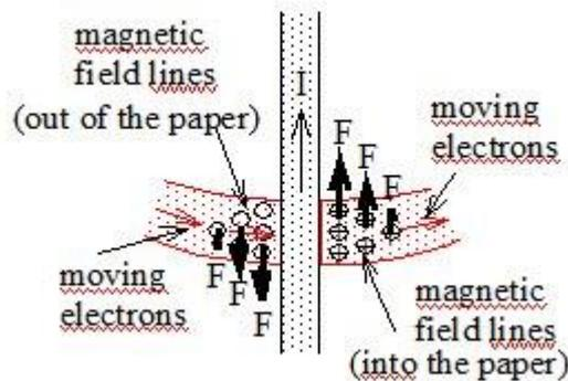
**Figure 5.** Magnetic forces on a current-carrying solenoid due to the magnetic field of a traversing external current.
