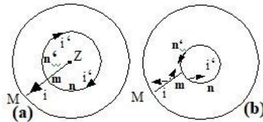
**Figure 9.** (a) The arrows indicate the tangential microscopic current  $i'$  of the magnet and the radial macroscopic current  $i$  flowing outside the magnet.
