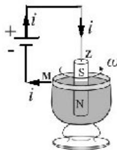
**Figure 6.** (a) A schematic representation of Ampère's motor
