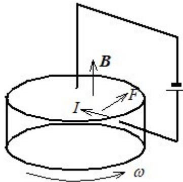
**Figure 2.** Schematic representation of magnet and circuit together with an indication of the magnetic force  $F$ .
