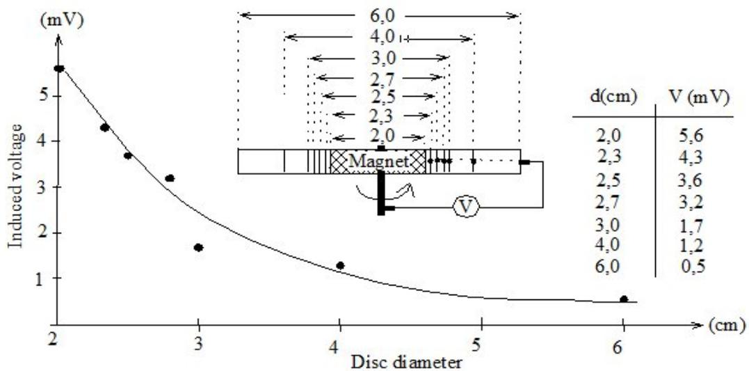
**Figure 7.** Measurement of the inductance voltage on ring-shaped aluminum discs, which rotate together with a magnet inside around a fixed axis
