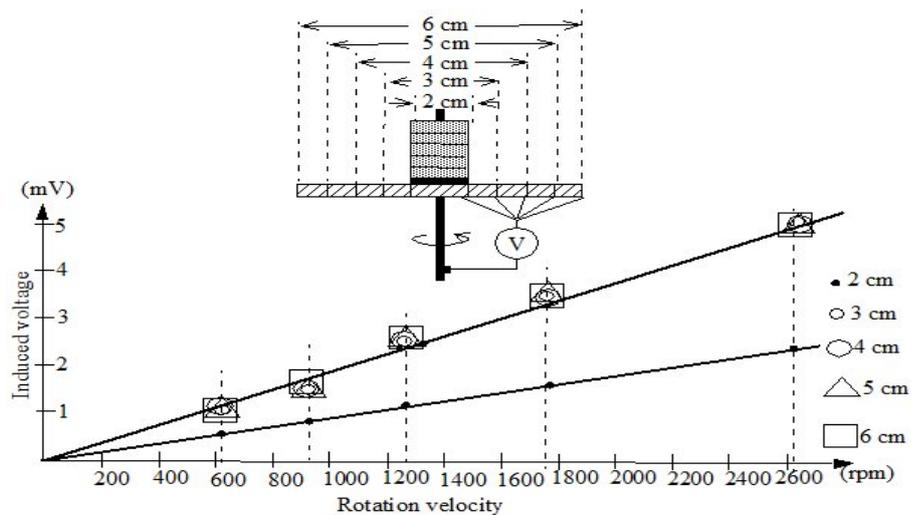
**Figure 4.** Induced voltage as a function of the rotational speed for different sized discs
