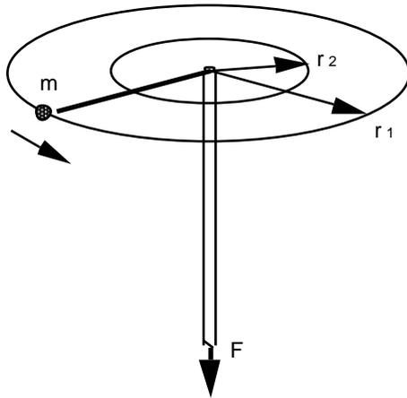
Fig. 1. An object attached to a string is set into motion in a horizontal plane. The string that is passing down through a hollow tube is pulled down to decrease the radius of rotation
