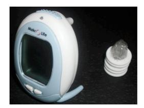
Figure 2. Audible thermometer
