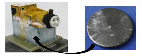
*Figure 2: The completed levitation train model with the nitrogen tank, and the toy train model placed above it. The melt-processed superconductor disk is placed in the center of the tank*
