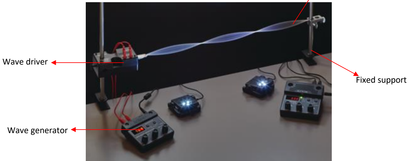
Figure 4: Suggested experimental set up. Image taken from https://www.pasco.com/products/lab-apparatus/waves-and-sound/ripple-tank-and-standing-waves/wa-9867
