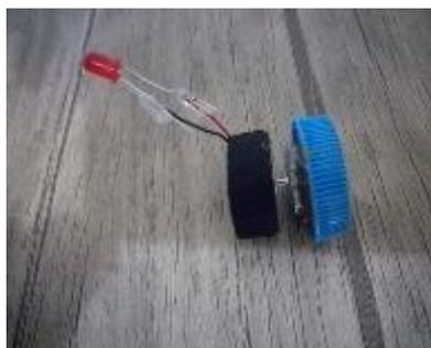
Using a motor with more voltage than the simple motor above, it was mounted on the wheel of the bicycle, and with the rotation of the bicycle, the blue cap began to rotate, so an induction field began to form, and the bulb gave light when the field was cut off.
