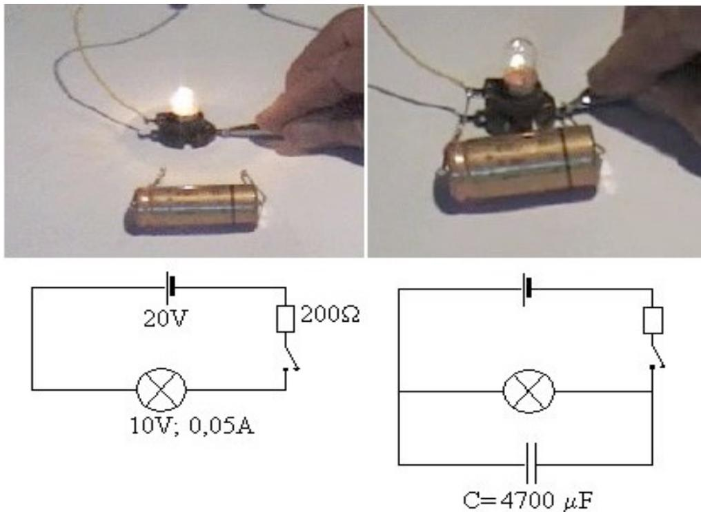
**Figure 2.** Demonstration of a Transition Process. A light Bulb is Connected to a Voltage Source directly or with a Capacitor Connected in Parallel.
