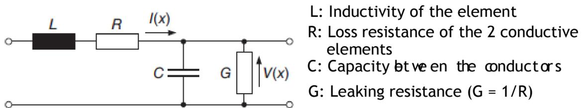
**Figure 5.** Model of an Element of a Twin Line
