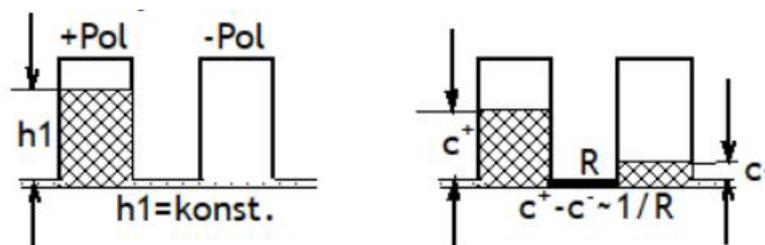
**Figure 9.** Model for a Battery (Left) and Resistor  $R$  with Two Connections (Right)
