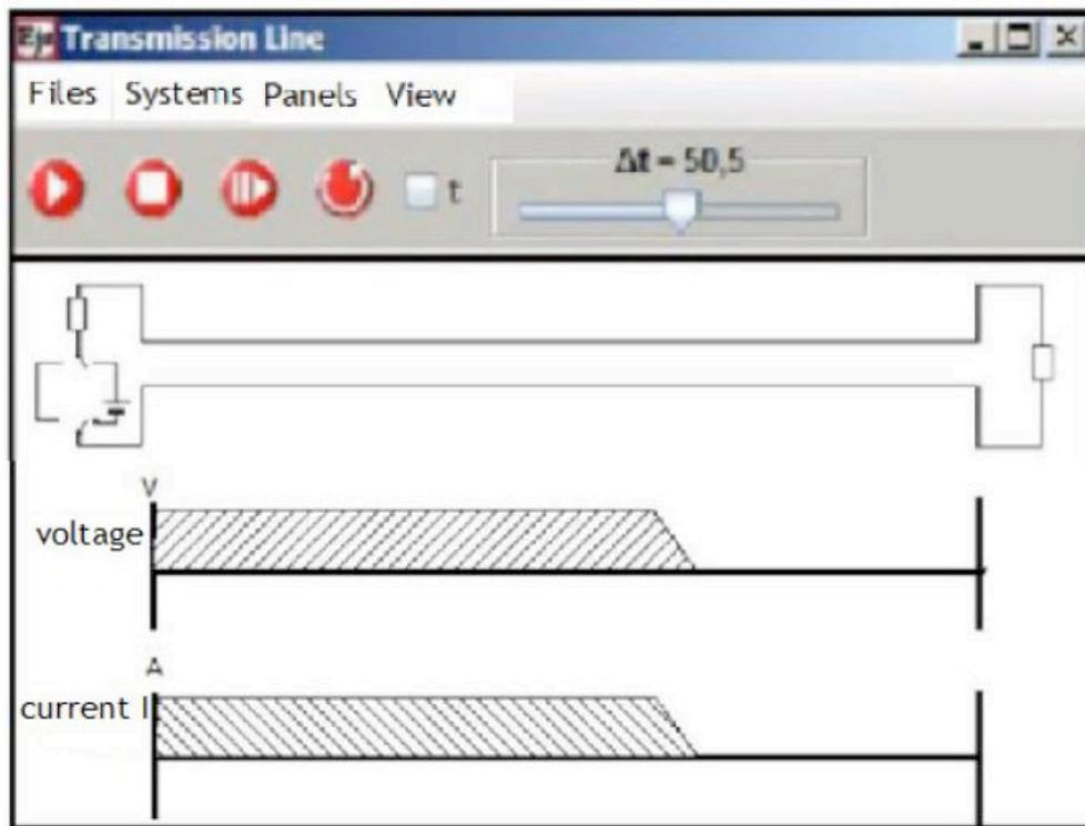
**Figure 4.** Transition Process After Connecting a Voltage Source to a Twin Line
