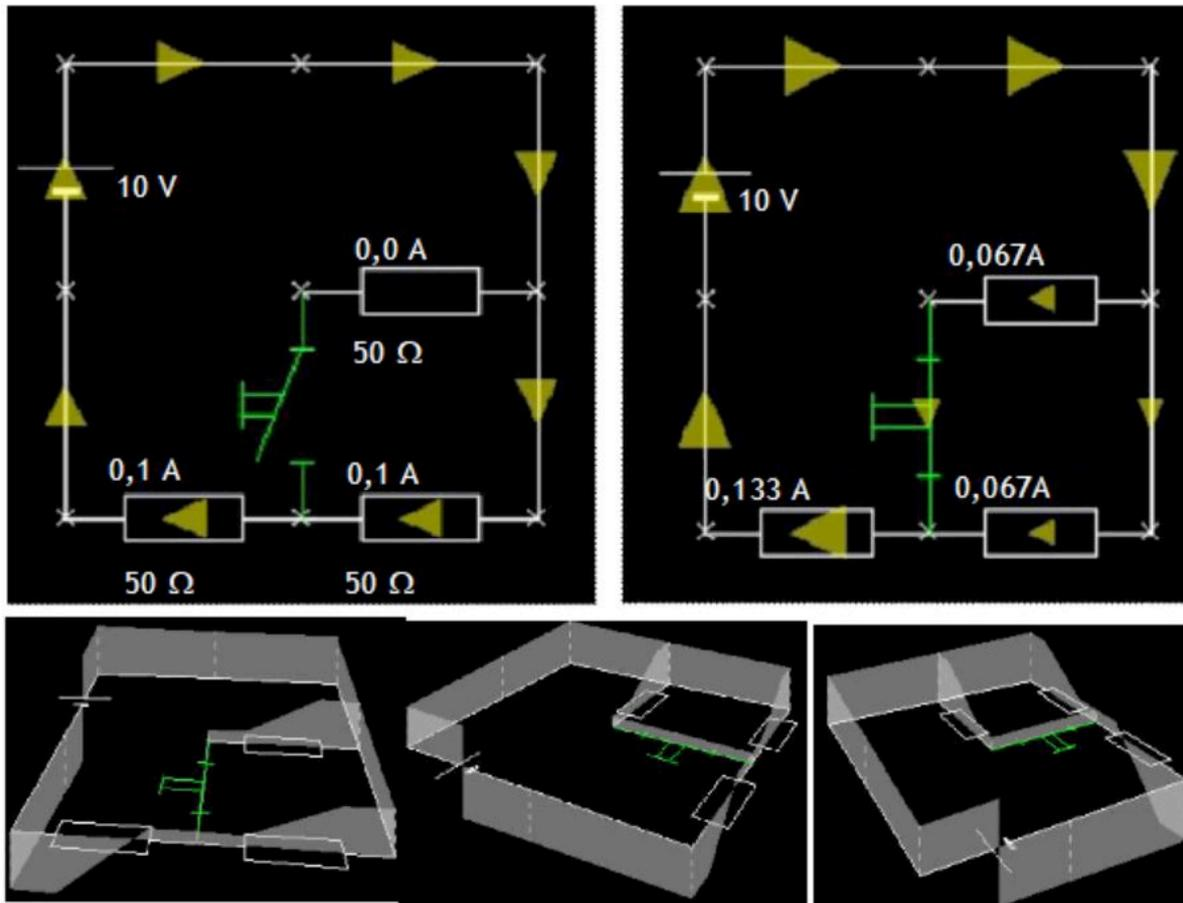
**Figure 3.** Screen Displays of the Simulation Program CLOC (See text). The Separate Window Showing the Circuit in 3D Can Be Rotated continuously.
