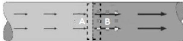
**Figure 5.** Application of Gauss Law at the Interface between a Conductor and a Resistor
