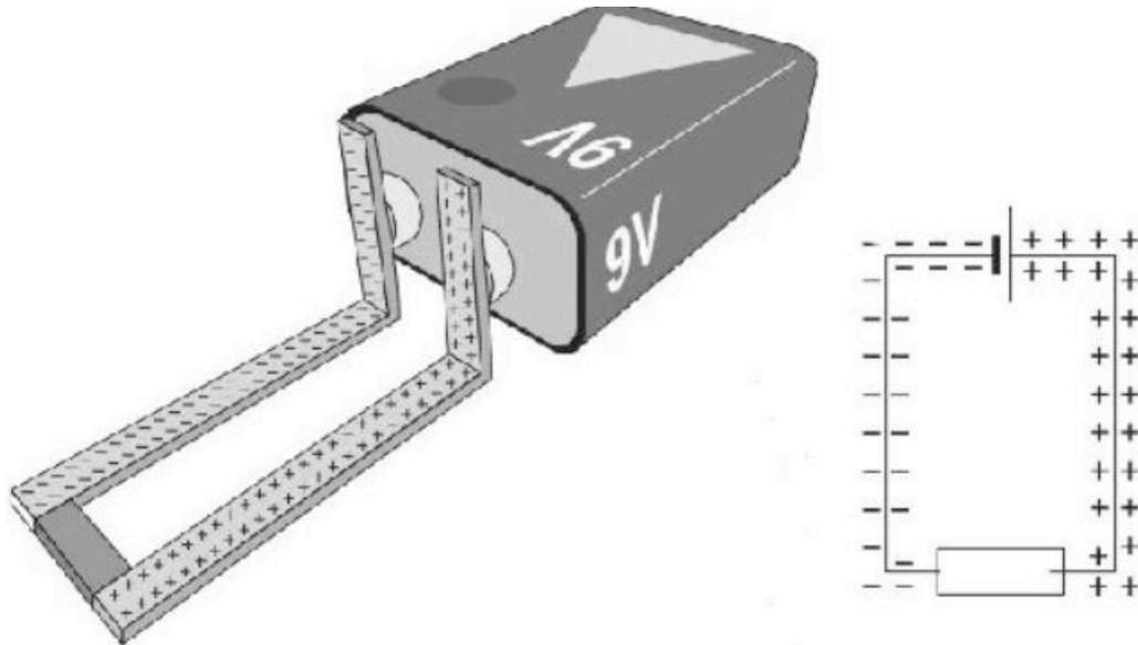
**Figure 10.** A Closed Circuit and Surface Charges
