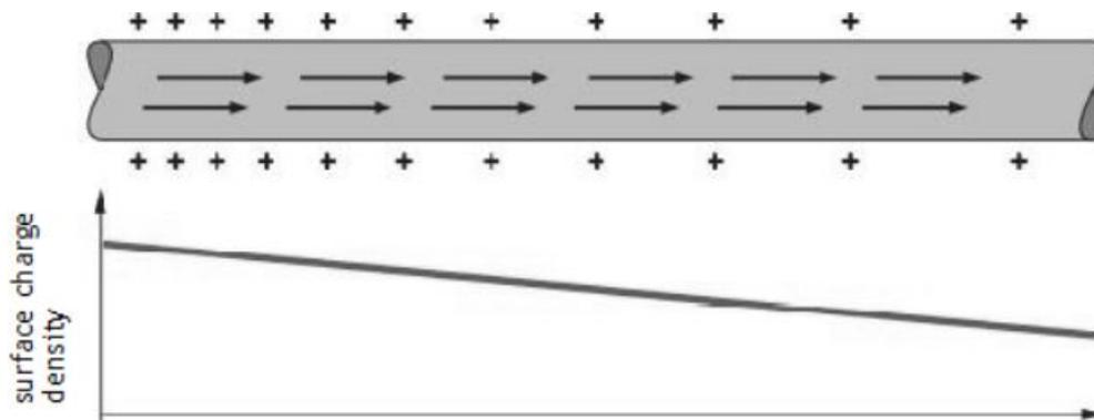
**Figure 6.** Linear Gradient of the Surface Charge Density
