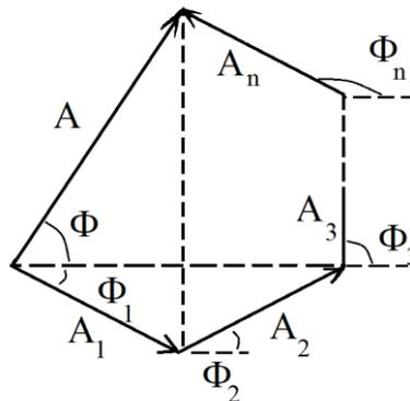
**Figure 5.** Multipath interference
