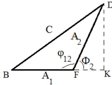
*Figure 1. Triangle with given sides  $A_1, A_2$  and the angle between them  $\varphi_{12}$*
