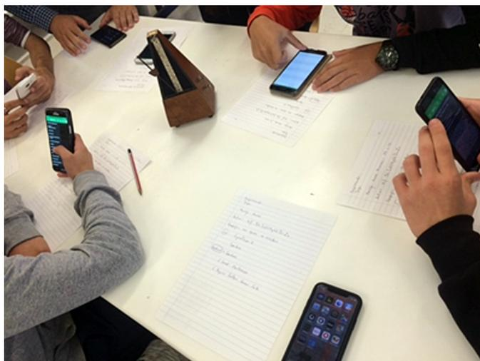
**Figure 5.** The layout of MPs around the metronome in order to measure the time between a certain number of strokes of the metronome
