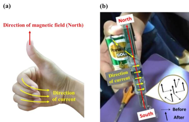
**Figure 2.** Underlining principle of magnetization. (a) Right-hand grip rule to determine the direction of magnetic field on the axis of circular coil carrying current. (b) In the vicinity of magnetic field, the dipoles of material were aligned in the same direction thereof.
