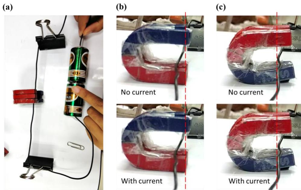
**Figure 3.** A schematic of the setup used for classroom demonstration of magnetic force, together with its corresponding results. (a) Experimental setup. (b) Magnetic force led the wire to move inside. (c) In contrast, magnetic force led the wire to move outside after reversing the horseshoe shape magnet.
