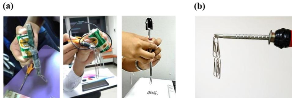
**Figure 1.** A schematic of the setup used for classroom demonstration of magnetization, together with its corresponding results. (a) Temporary magnet could be turn on and off by controlling the electricity. (b) Permanent magnet continually attracted the objects after magnetization.
