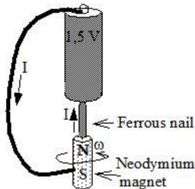
*Figure 1. The "simplest" motor*
