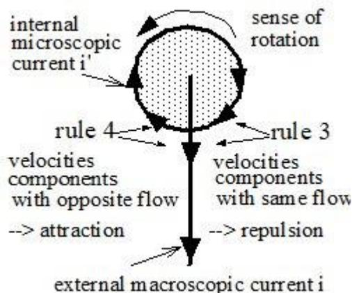
**Figure 10.** Exemplification of Ampère's explanation of how his motor works
