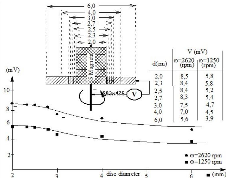
**Figure 8.** The same measurement as in Figure 6 with a more giant, more extended magnet
