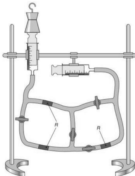
**Figure 12.** Rearranged Syringe Model to Measure the Current
