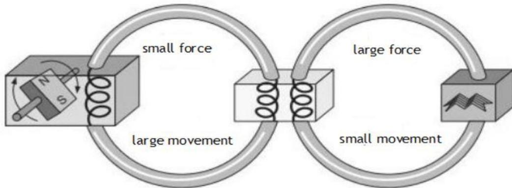
**Figure 9.** Symbolic Representation of an AC-Current Connected to a Transformer
